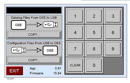
Successful password entry gains access to the main Configuration Menu as soon as the last digit of the correct password is pressed. The '**CLEAR**' button can be used to clear an errant entry before retrying. Any incorrect or incomplete entry will be cleared automatically if 5 seconds elapses without any input or if the '**EXIT**' button is pressed.
