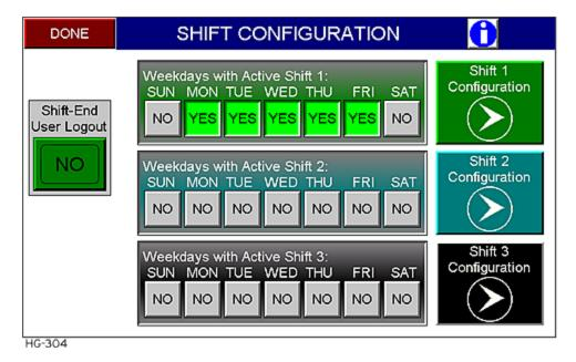
For each Shift, select the days of the week with an active Shift on this Work Cell. Configured shifts will start and end automatically on these days. These active days are mirrored within each separate shift configuration screen.
