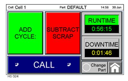
Add Cycle: For Touchscreen cycle triggering, the green Add Cycle button will trigger a single cycle each time it is pressed.
