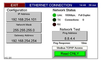
The IP address configured here is normally how the Data Concentrator will know how to find this work cell. This may not be true of advanced networking through routers, firewalls, cell modems, etc.
