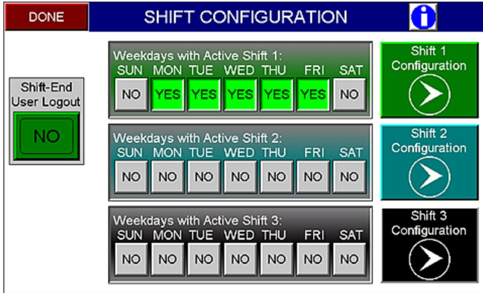
For each Shift, select the days of the week with an active Shift on this Work Cell. Configured shifts will start and end automatically on these days. These active days are mirrored within each separate shift configuration screen.
