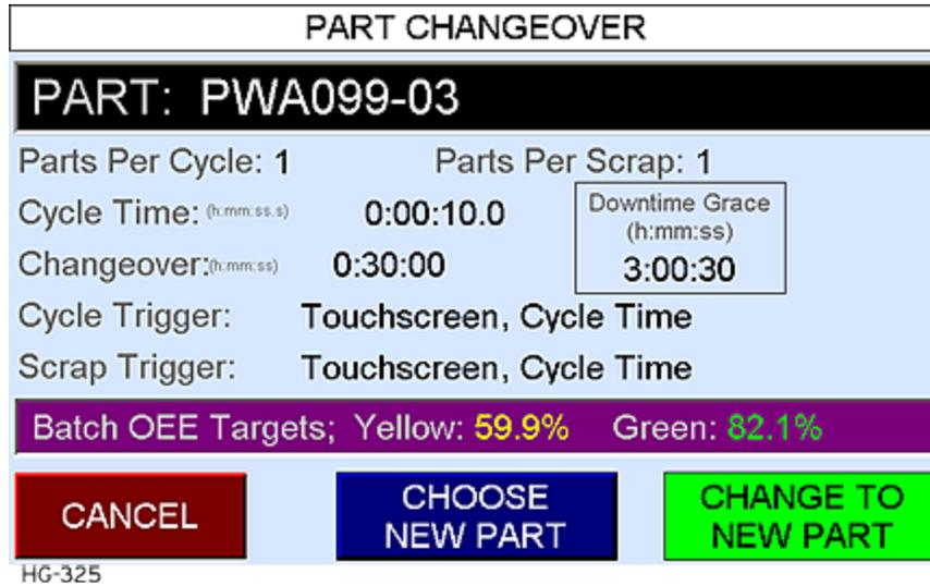
Selecting 'Choose New Part' will present the user with a directory of available parts from which to select. The MicroSD card must be in place for this operation to be available. These part files are created using the Part Editor/Viewer in the Configuration menu or by using the Configuration Utility.
