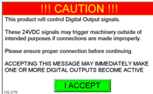
No outputs will become active until this CAUTION message is accepted. Please refer to wiring diagrams and be sure to fully understand the intended connections before accepting this message.
